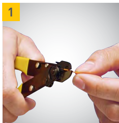
Remove the sheath from the fibre
